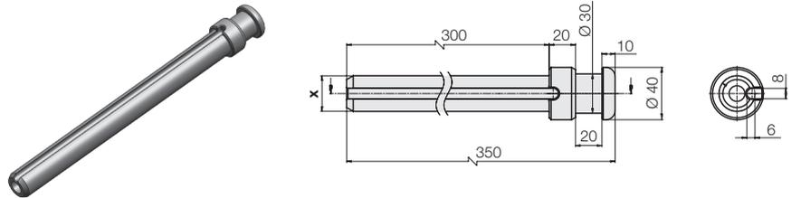
Abmessungen in [mm]
