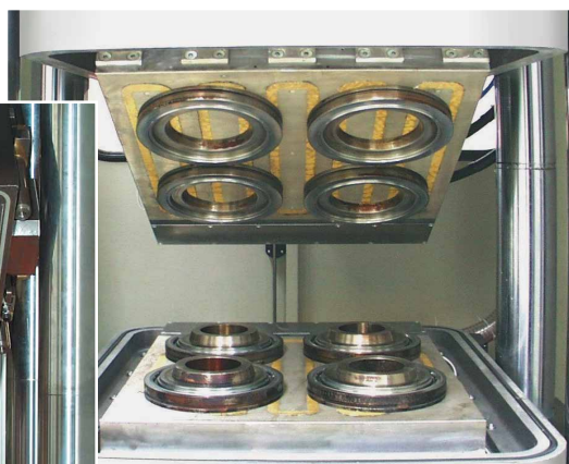
M-TECS R on a vertical press - various moulds on a machine bed without loss of space due to clamping claws
