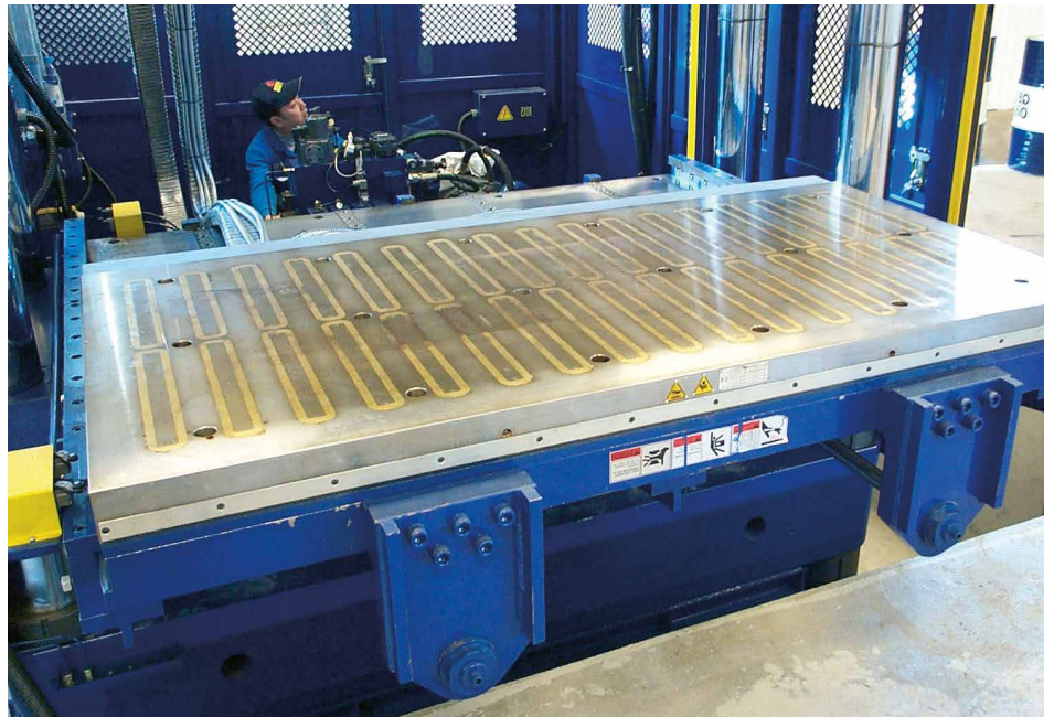
Magnetic clamping system on a vertical press for temperatures up to 240 °C
