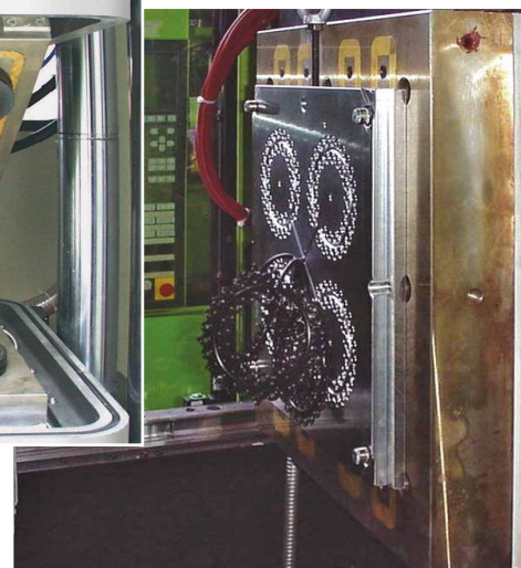
M-TECS R magnetic heating plate on an elastomer machine - full-surface magnetic force gives full-surface contact and more homogeneous temperatures
