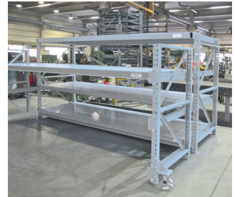
Die storage with laterally retractable side guides
