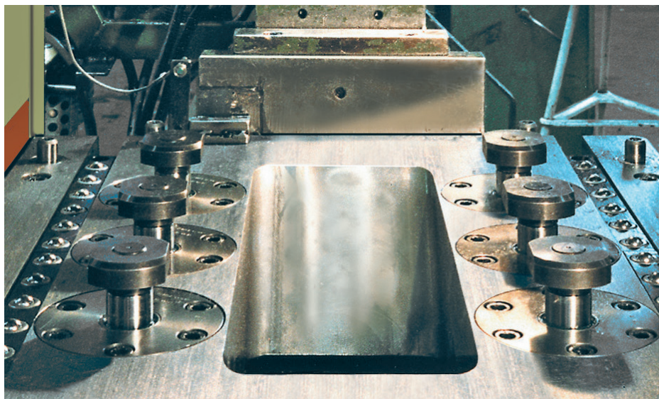
Pull clamps in the press bed of a double-column press.
