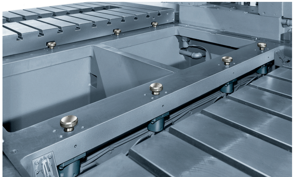
Clamping of a die changing table with pull clamps
