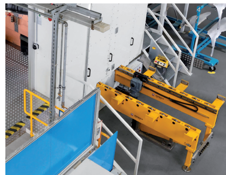
Die changing console with drive and side loading of the press.
